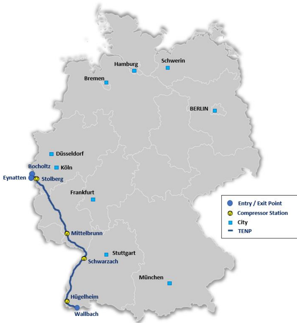
Figure 3: The route of the TENP pipeline, entry and exit points and the compressor stations along the pipeline.
